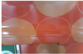
< Failure of V drawing >
